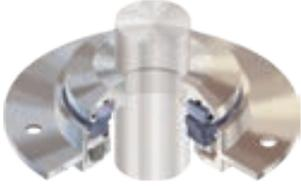
The GLS is the liquid service configuration of the Flowserve GSS. It is designed to fit the unique installation envelop and operating speeds present in integrally geared pumps.
